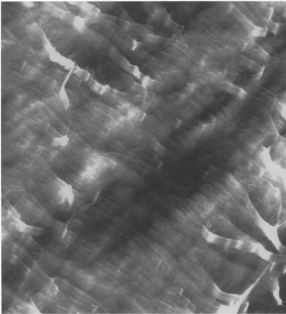
Figures 1a - 1c: AFM height images at different places. Fiber orientation is indicated by an arrow. Scanning areas: (a) 3.65 \times 3.65 \mu^2 • (b) 2.05 \times 2.05 \mu^2 • (c) 4.08 \times 4.53 \mu^2 • A gray scale contrast spans over 100 nm height variations.
